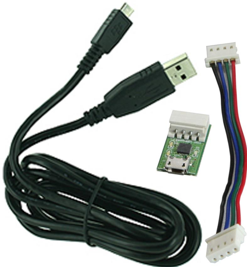
Assemble the USB-UART module and cables as shown in this picture.
