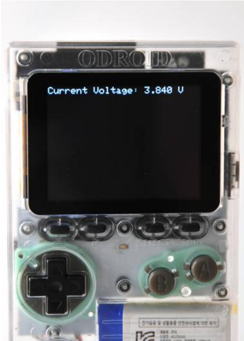
ODROID-GO has a ~3.7V battery module.
