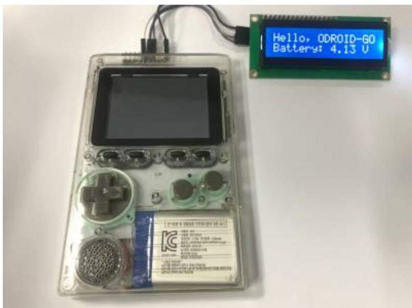
We have prepared more an advanced example based on the previous we made together. Click the **Files** → **Examples** → **ODROID-GO** → **16x2\_LCD\_I2C** menu to import and press **CTRL-U** to compile/upload.
