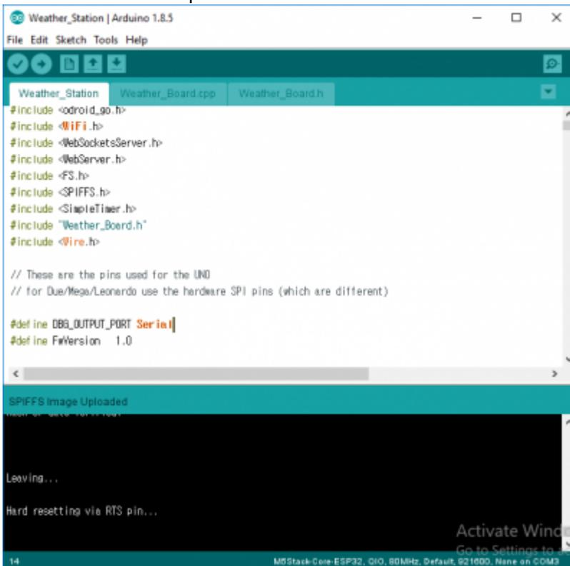
The uploading is complet when the message "Hard resetting via RTS pin..." is displayed.
