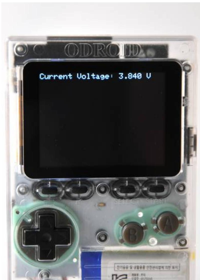
ODROID-GO has a ~3.7V battery module.
